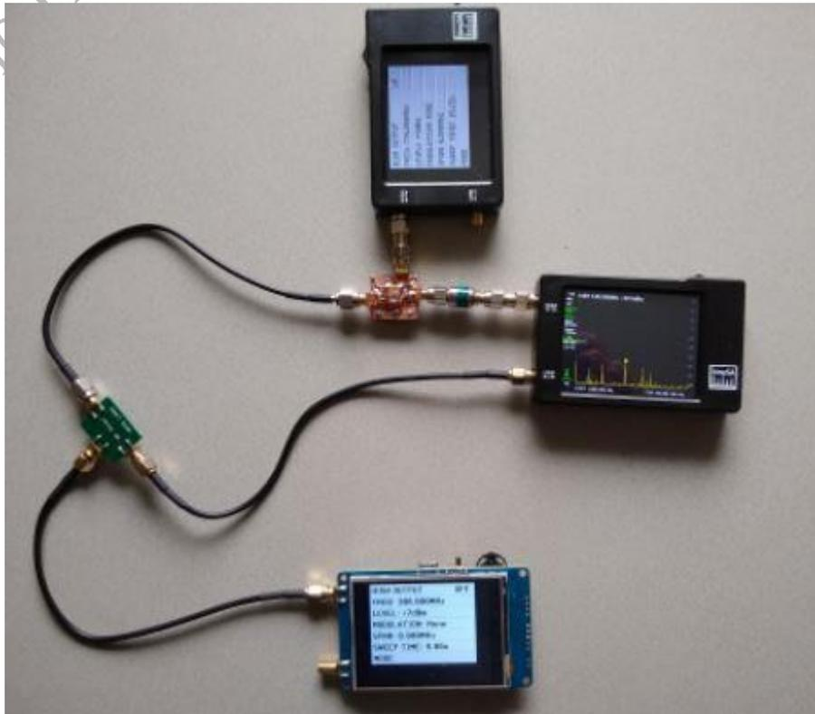
In the lower left corner there is a green module with the mixer to be tested. The LO output of the TinySA on the right is used as an input to a copper foil-coated mixer via a 20dB attenuator to create a tracking generator. The tiny SA at the top is the LO of the TG mixer. The tiny SA at the bottom is the LO of the mixer under test
