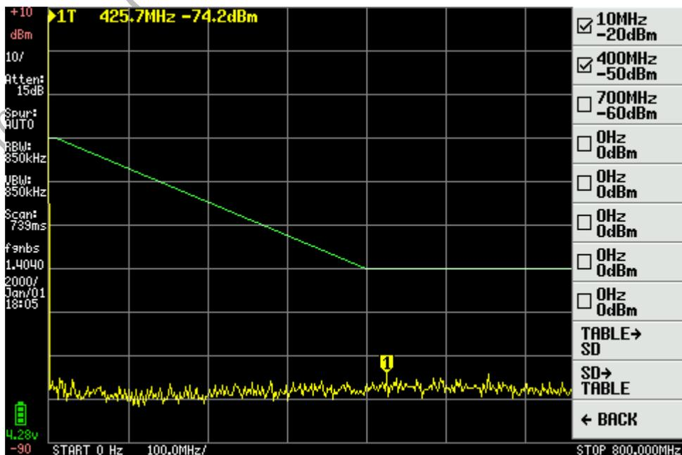
There will be a horizontal line from zero Hz to the first active entry, and a horizontal line from the last active entry to the end of the scan range.
