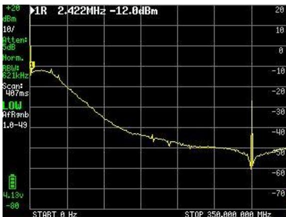
It turns out that the output impedance of the mixer under test is not matched correctly.
