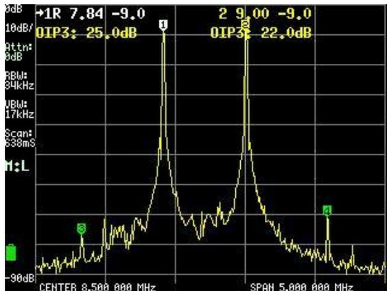
When we increase the tiny SA input attenuation to 5dB, the intermodulation product on the left disappears, so it is generated internally. The correct intermodulation product does not change, so it is present in the input of TinySA
