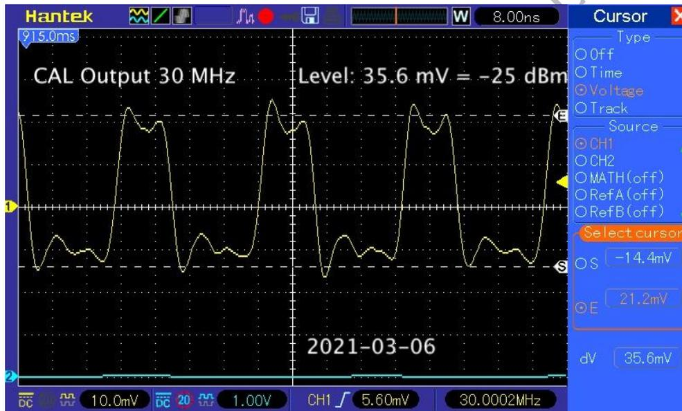
Small deviations can be explained by the harmonics present in the calibration output.
