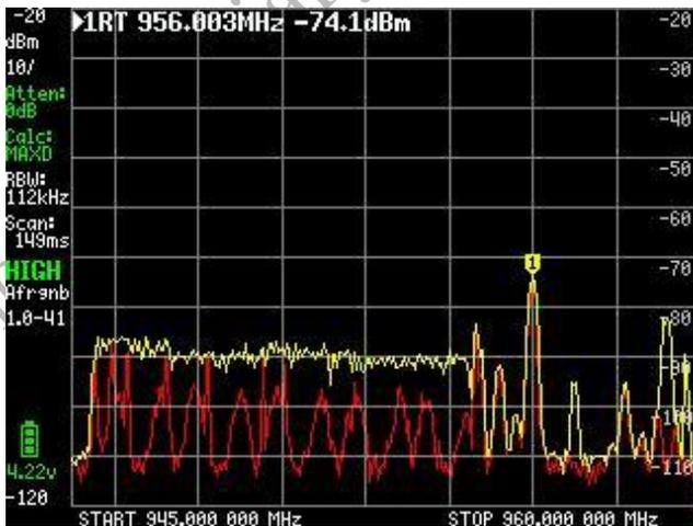
The signal below the power envelope and markers increased by almost 20dB
