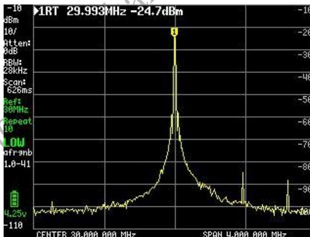
Since the sample is repeated multiple times to measure each point, there is some delay in between, and the scan time will increase
