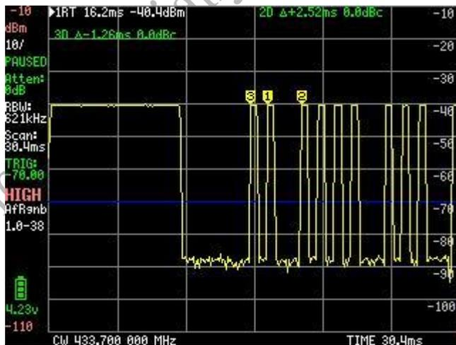
Using the marker in incremental mode, the discovery bit timing is 1.25ms
