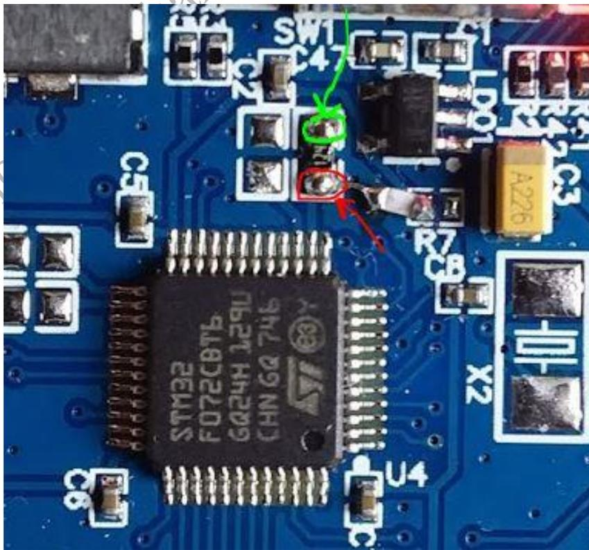
The ground of the audio output circuit can be connected to a pad with a green circle or any other GND PCB edge pin.
