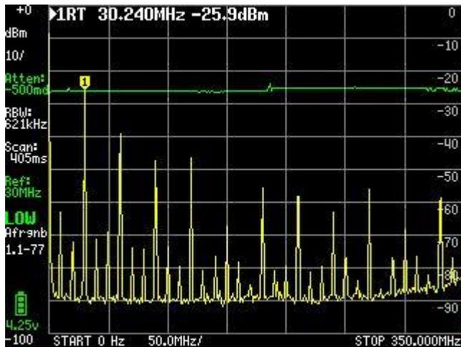
If you observe a deviation of more than +/- 1dB in the green line (excluding some noise/interference), please post a readable picture or screenshot of the completed linearity test on the TinySA support group
