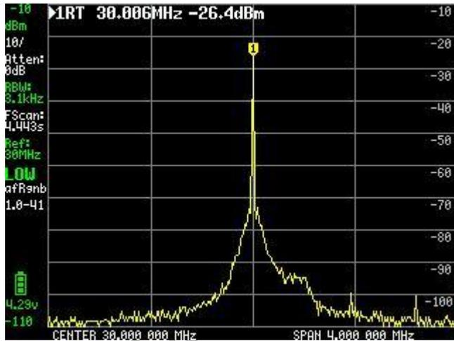
Again, about 3 times faster than a normal scan with a 4kHz RBW
