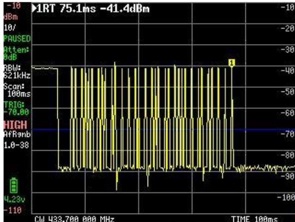
After a single trigger occurs, the status changes from "armed" to "suspended"
