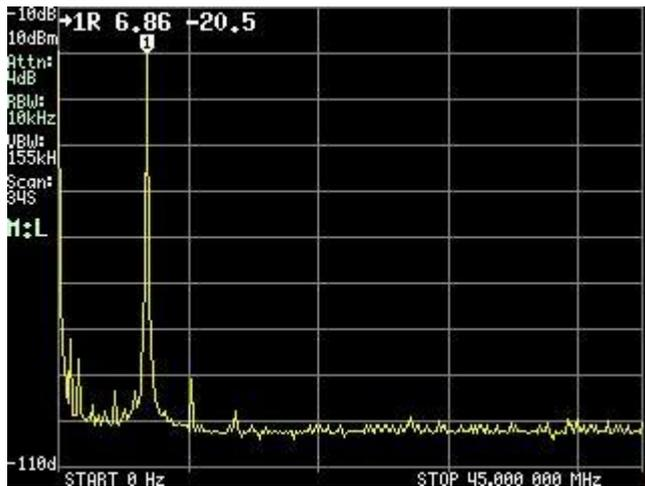
When the level of the second harmonic moves downward, it is generated internally. With this 2dB attenuation, the second harmonic is now below -4dBc, which is the maximum SFDR for TinySA.
