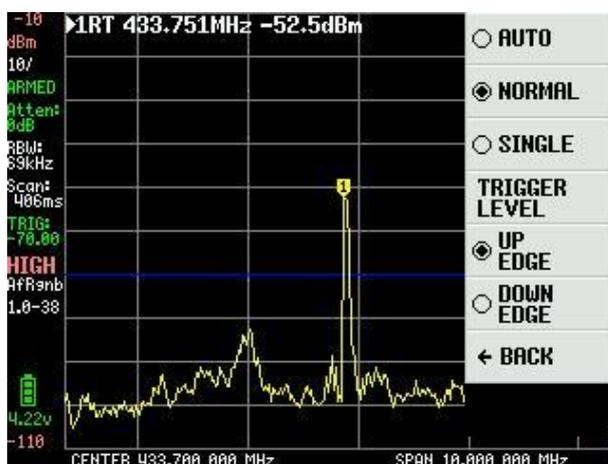
You can see in the status panel that the trigger is armed, so any new signals are automatically displayed
