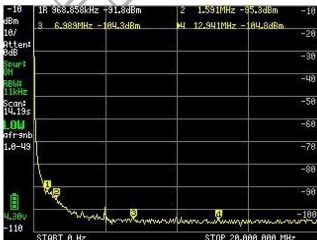
This results in an almost clean noise floor. To check if the same scan has no effect on sensitivity
