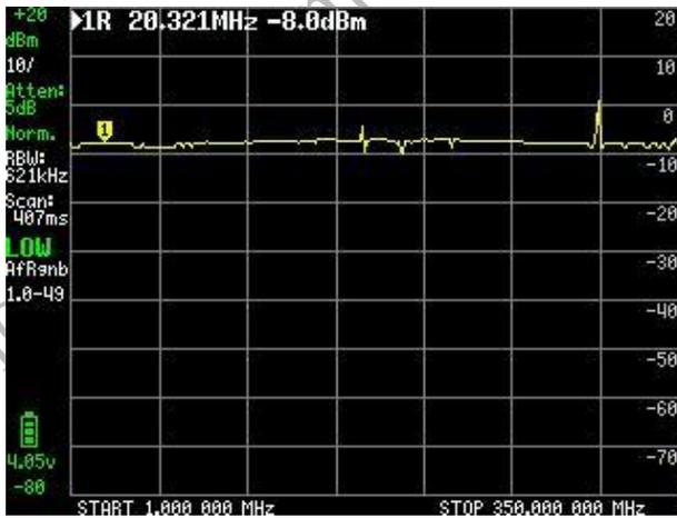
The loss is about 8dB, which is well within specification.
