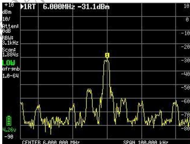
This strange effect of many signals is caused by a completely failed internal AGC. You must ensure that the level of the input signal carrier minus the internal attenuation is below -45dBm by manually increasing the attenuation.
