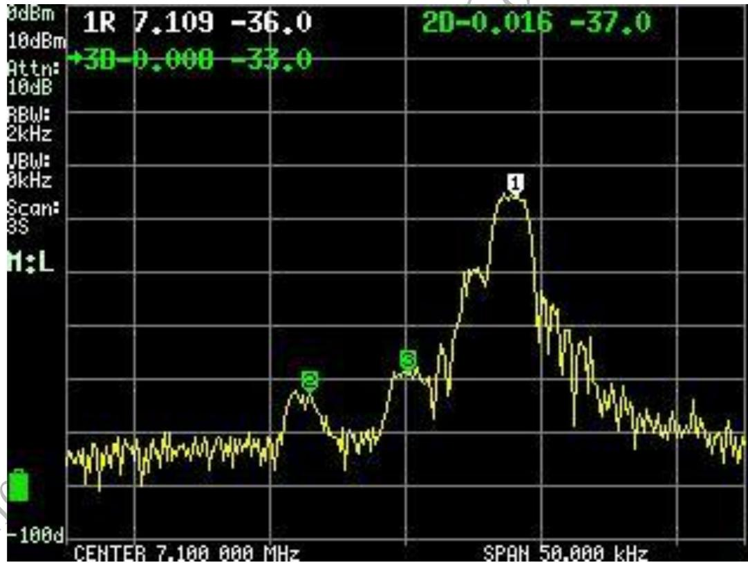
Adjust the IQ balance a bit to divert unwanted sidebands to noise below -40dBc
