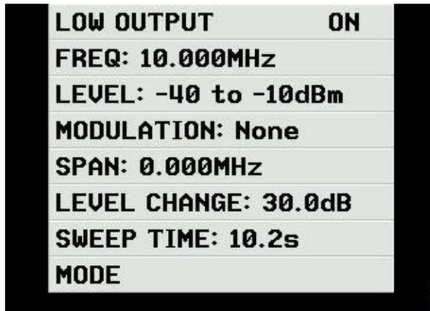
The frequency is 10MHz and the output level changes from -10dBm to -2dB in 40.10 seconds. The output of the generator is connected to the input of the amplifier, and the output of the amplifier is connected to another tiny SA. The second TinySA is in low input mode, set to zero-span mode at 10MHz, with a scan time of 10 seconds and a normal drop trigger of -10dB level as shown below.
