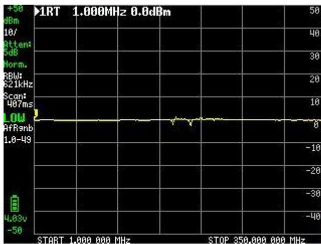
Then plug in the mixer under test as shown in the first image and set the TG to offset to 734MHz, resulting in a 300MHz offset
