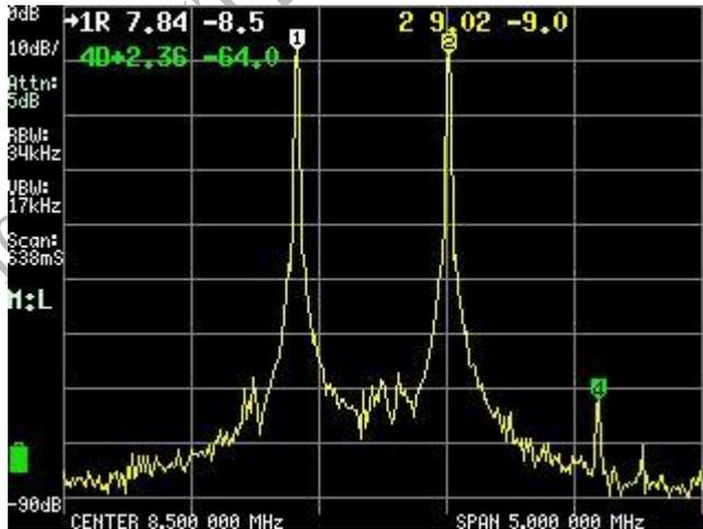
Now that we know the IIP3 of the TinySA, we can start measuring the IIP3 of the amplifier. First, we use two tiny SAs to create a two-tone generator. These are the two tone outputs including harmonics.
