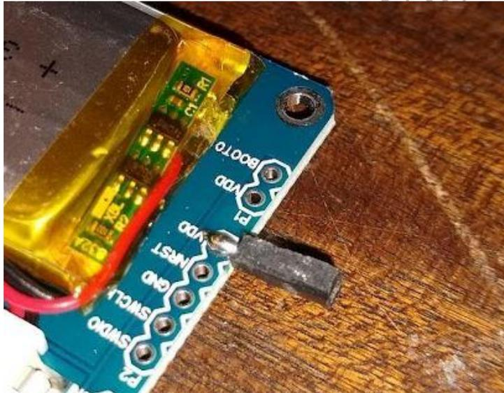
Warning: The maximum current consumption is 100mA. Monitor the temperature of the tiny SA and turn it off if it's hot. Drawing too much current can ruin your tiny SA
