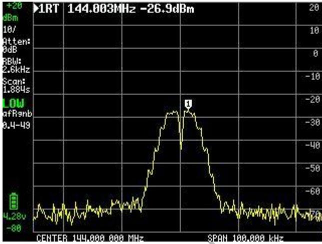
Using a deviation of 11kHz you get the next bessel zero
