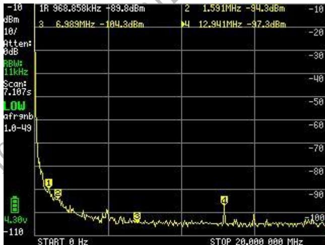
TinySA has an internal table that records at what frequency the IF must move to eliminate some of the spurs. This method of avoiding irritation has no negative impact on performance.
