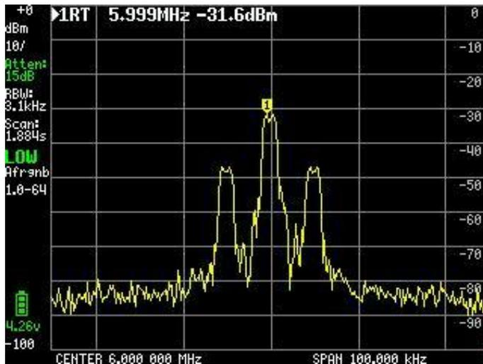
The lower limit of modulation that can be observed in frequency mode is indeed 3kHz at a minimum RBW of 3kHz
