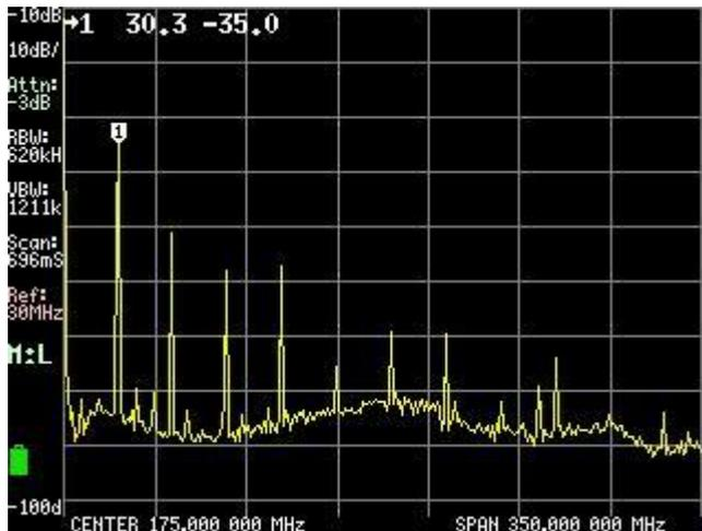
The fundamental frequency is 30.3MHz and the intensity is -35dBm
