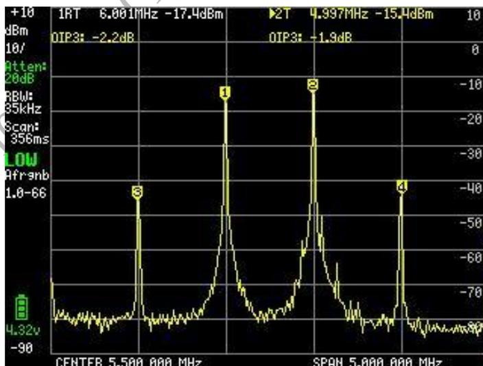
Since the signal level we observed was 3.5 dB lower, because without the amplifier and attenuator, we would have to add 3.5 dB to the measured IIP3, which is about -2 dBm, so we get +3.1 dBm of IIP5 amps. It's 6.5 dB lower than what we measured without the amplifier and attenuator, so we can be sure that we're measuring the IIP3 of the amplifier.
