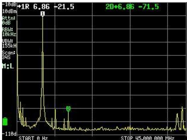
And add a little attenuation to check if the remaining second harmonics are produced internally.
