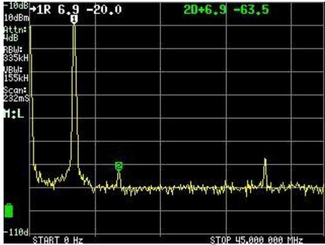
A low-pass filter is inserted between the transmitter and the TinySA to eliminate the second harmonic, and in effect it disappears into the noise
