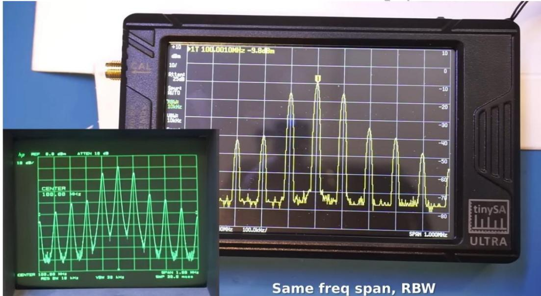
The results of the TinySA and benchtop frequency meters are very consistent
