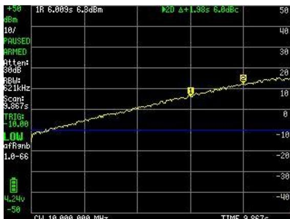
Then move the marker to the right to a position where instead of adding 3dB per half, only 2dB is added.
