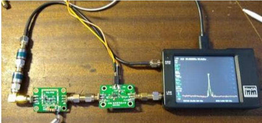
We can read the amplification (36.8dB) of the cascade amplifier directly below the marker
