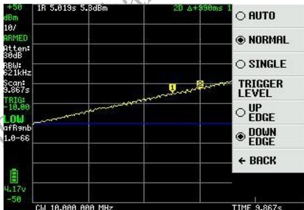
When the signal generator jumps back to -40dB, the second TinySA triggers and starts recording the level for 10 seconds. Using two markers (a reference and an increment marker), it is easy to see that the level increase for each cell is 6 dB (5 cells, 30 dB total).
