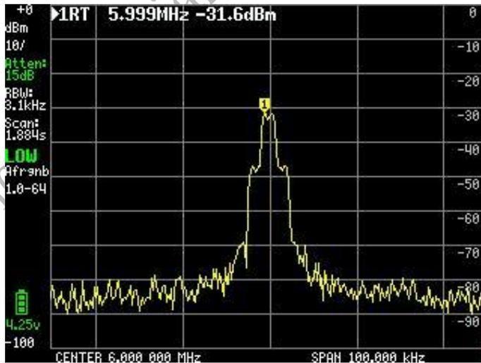
For lower modulation frequencies, it is advisable to enter a zero-span mode (time mode) and a linear unit to show the signal strength as a function of time, where 50% of the modulation depth can be clearly observed
