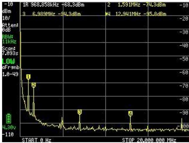
The first measure used is to move the IF at certain scan frequencies. When the IF is set back to automatic, the impact is clearly visible.
