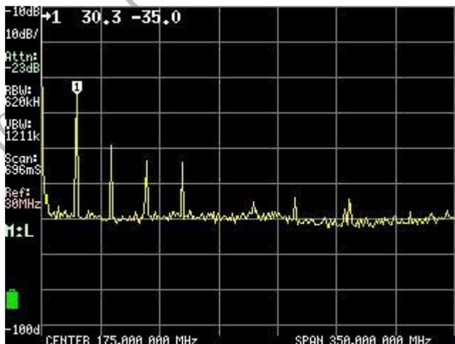
As shown in the figure above, if harmonics remain at the same level as the attenuation increases, it can be determined that these harmonics are not generated internally, but are present in the input signal. When the harmonics decrease in intensity as they increase the attenuation, you have overloaded the TinySA and the harmonics (partially) are generated internally
