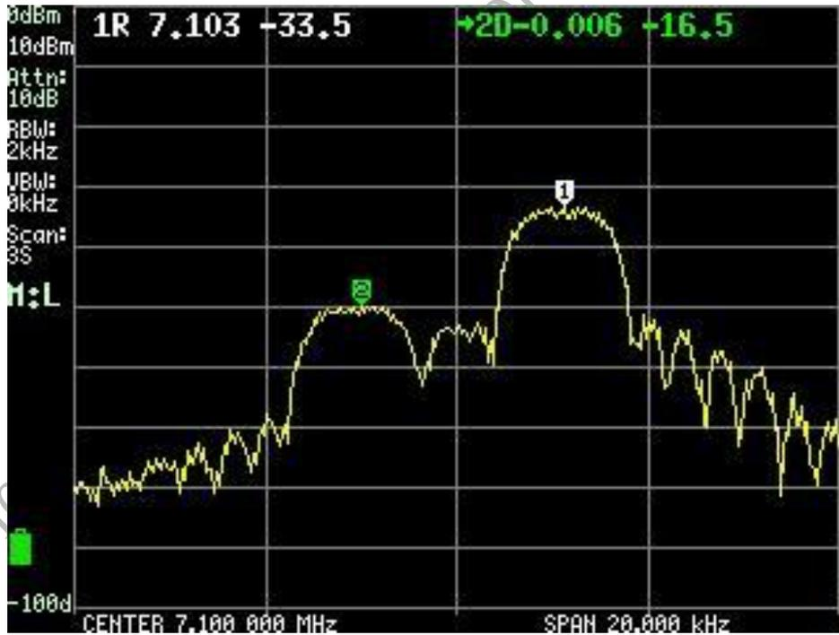
Marker 1 is the required USB and Marker 2 is the LSB that is not needed
