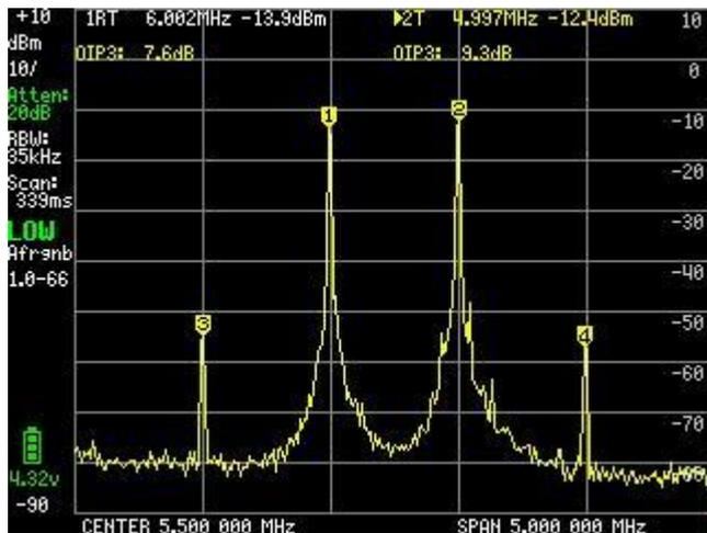
The OIP3 of this dual tone generator is about 8 dB, so we had to carefully create a test setup to make sure this doesn't hide the amplifier IIP3.
