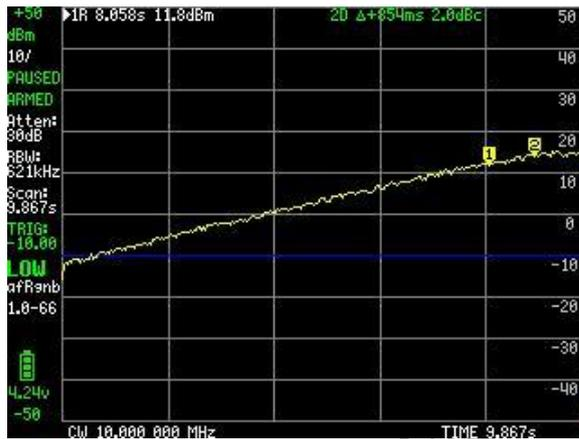
The amplifier's output 1dB compression level is 13.8dBm at mark 2, and the amplifier's input level of -40dB plus 9 times 3dB (or -10 minus 3dB) at that point equals -13dBm. Keeping the amplifier's input below -13dBm will ensure no compression.
