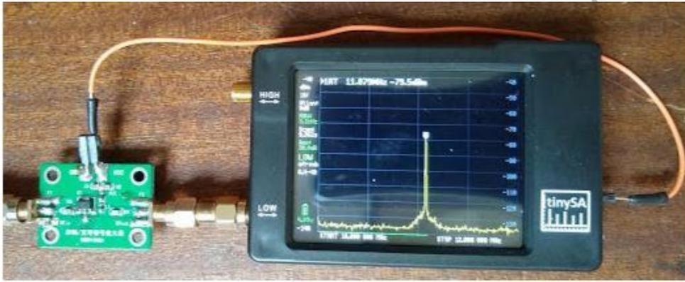
Combined with a small telescopic antenna, the TinySA is ready for some QRM hunting
