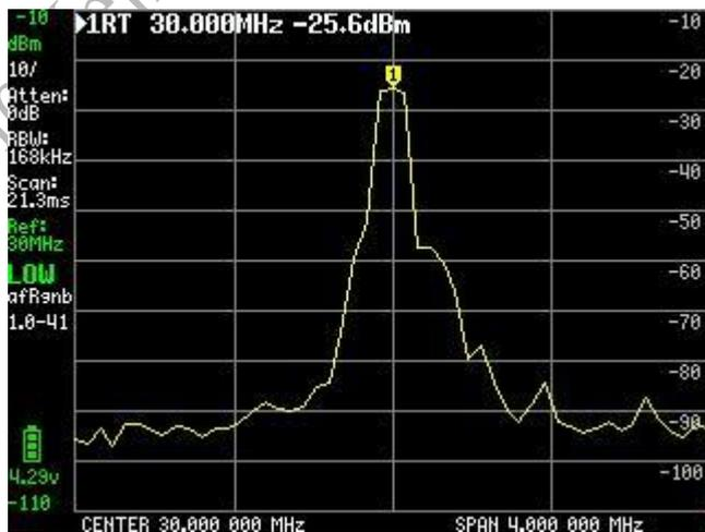
Notice reducing the number of points increases the automatic RBW selection from 28kHz to 168kHz but reduced the scan time to only 21ms. Ideal for tuning some circuit or filter
