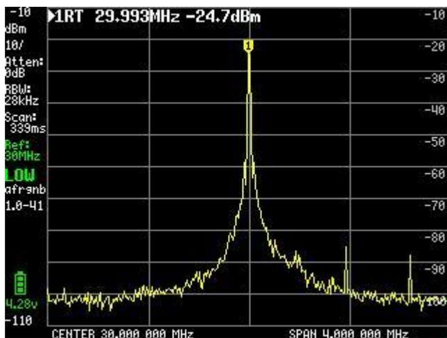
The important number to note is the indicated scanning time. In this case, it's 339 milliseconds. Sometimes small signals can be seen, and enabling SPUR removal will help identify if these signals are real or not
