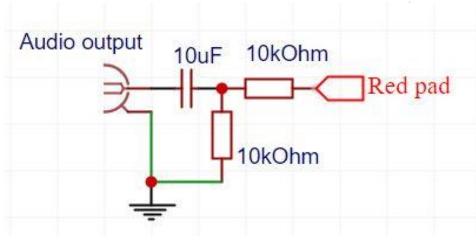
The headphones can be connected directly to the audio output. If you need volume, move the 10k to the ground and replace the remaining 10k with 4.7k
