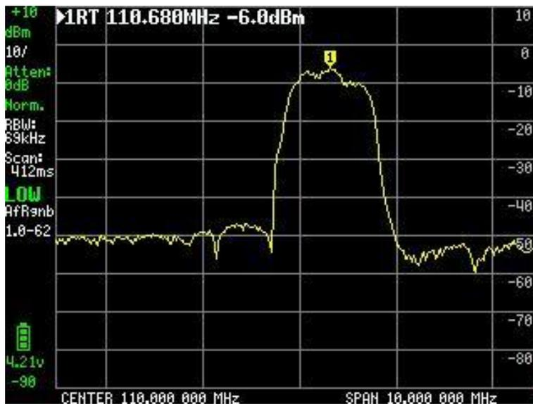
The dynamic range in this setup is limited due to the mixer's reverse leakage. It is a good idea to add an attenuator and amplifier between the LO output and the tracking generator input to stop leakage. If an external mixer is used, the conversion loss of the mixer can be measured by setting the TG to the offset.
