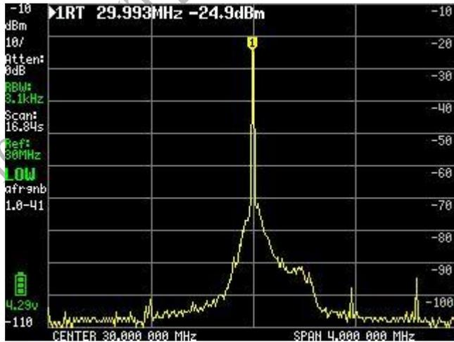
Note that the scan time is increased to 16.8 seconds because smaller RBWs need to measure more frequencies and take longer measurements per time.
