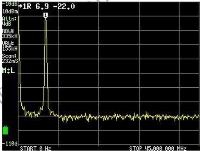
RBW is lowered to reduce the noise floor. The second harmonic is now visible again at -2.71dBc
