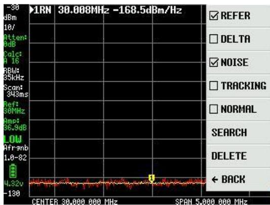
To calculate the noise figure of the first amplifier, we simply subtract -174dBm/Hz (noise power per hertz at a 50 ohm resistor at room temperature) to get a noise figure of 5.5 dB. The specs of the first amplifier give 4.5dB of NF, so we're close.
