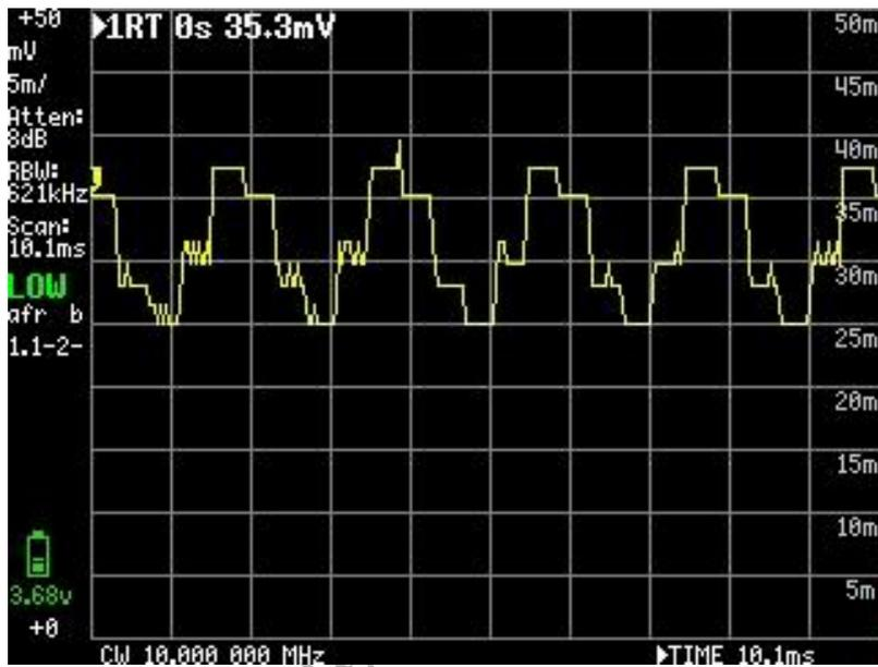
In external modulation mode, a second TinySA acts as a spectrum analyzer in low input mode and can drive TinySA's mixer in low output mode by setting the LO output to output its LO from its high connector. By setting the frequency to zero Hz, the output will follow the Spectrum analyzer with zero Hz offset and can be used as a tracking generator.
