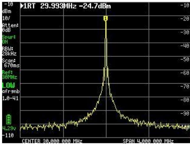
Since the small signal is no longer visible, these artifacts are created internally. Note that removing the SPUR doubles the scan time.
