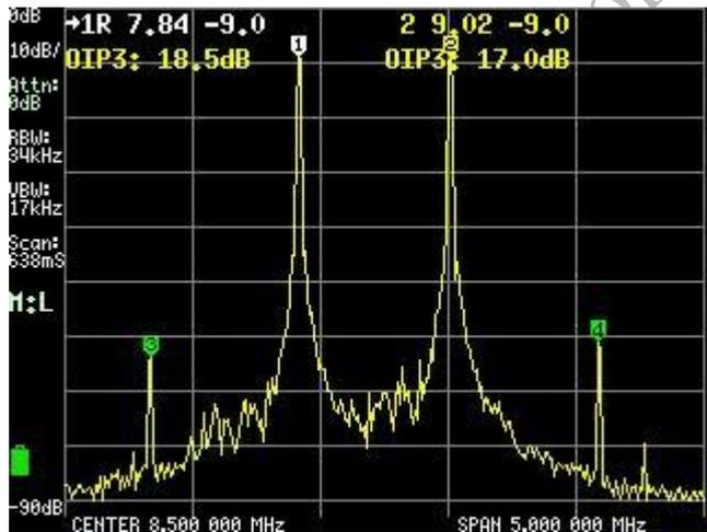
Attenuator settings are very important. At low attenuation, the tiny SA first mixer performance will most likely limit the maximum OIP3 that can be measured. Changing the attenuation amount should be noted to change the measured OIP3. If so, you should increase the attenuation until it is no longer so.
