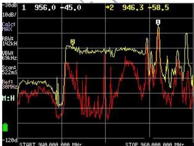
The graph above shows the power envelope of a cell phone base station traveling between 945MHz and 955MHz. The yellow trace is set to maximum hold, and the red trace shows the current transmit power.
