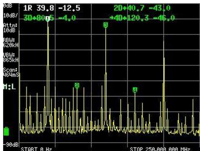
The difference between harmonics and aliasing and DDS is clearly visible.
